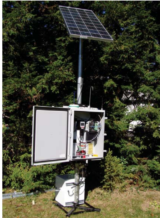
AirLogics SolarLite automated perimeter air monitoring system. Photo courtesy of AirLogics, LLC
