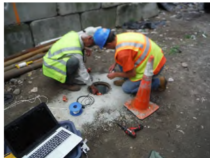
Photograph 36: Performing monitoring well slug testing. Date: September 7, 2017.
