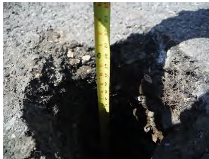
Photograph 14: Soil boring pre-cleared to 5 feet below ground surface. Date: August 15, 2017.
