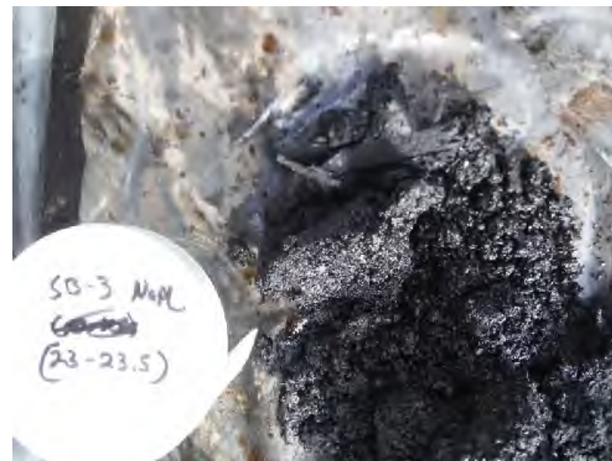
Photograph 16: NAPL (non-aqueous phase liquid) observed in soil boring SB-3 from 23 to 23.5 feet below ground surface. Date: August 8, 2017.
