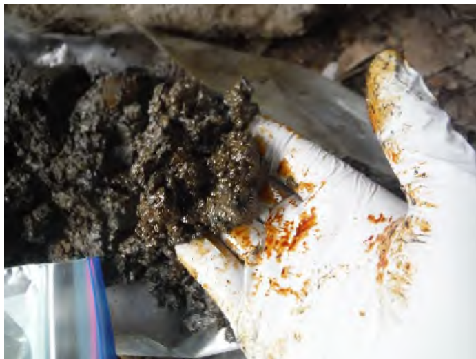
Photograph 17: NAPL observed in soil boring SB-1 from 17.5 to 18 feet below ground surface. Date: August 8, 2017.
