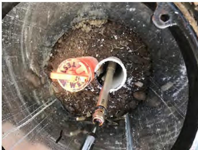
Photograph 37: Performing monitoring well slug testing. Date: September 7, 2017.
