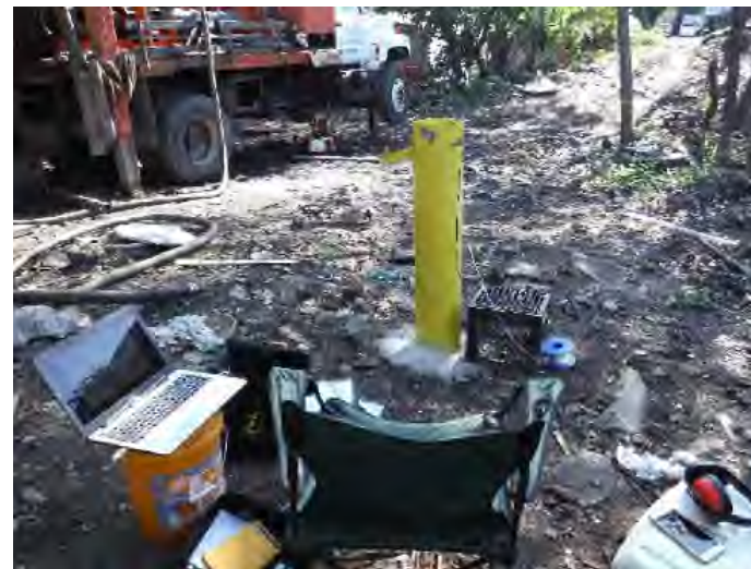
Photograph 38: Performing monitoring well slug testing. Date: September 7, 2017.
