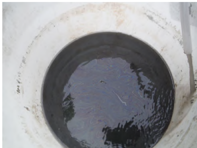
Photograph 27: Sheen visible on purged groundwater. Date: September 12, 2017.
