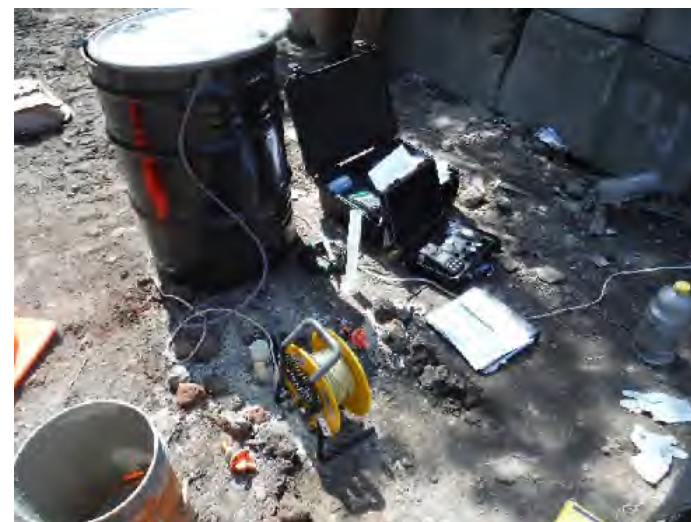
Photograph 24: Purging of monitoring well using low-flow groundwater sampling techniques. Date: September 12, 2017.
