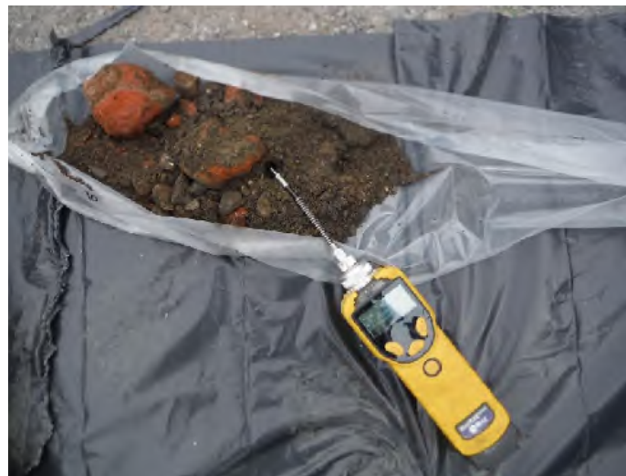
Photograph 18: Field screening soils with a hand-held photoionization detector (PID). Date: August 8, 2017.
