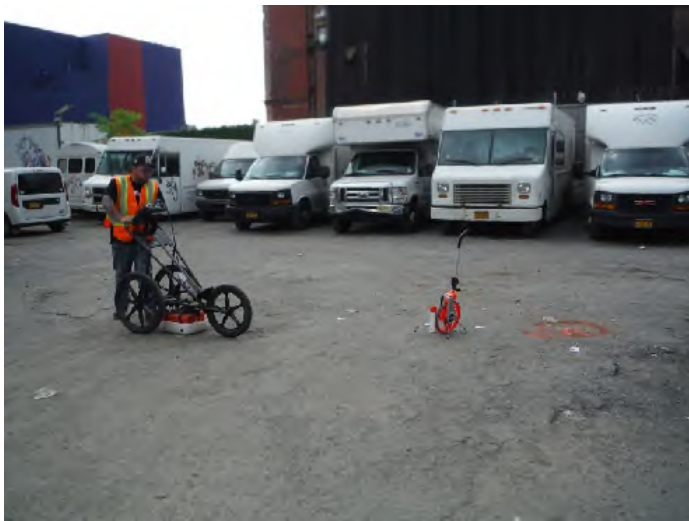
Photograph 11: Geophysical ground penetrating radar survey of the site. Date: August 15, 2017
