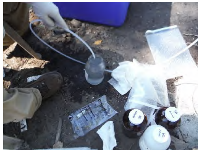
Photograph 28: Sampling of groundwater from a monitoring well. Date: September 13, 2017.
