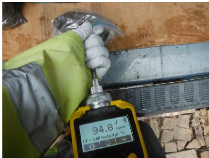
Photograph 19: Field screening soils with a hand-held PID Date: August 8, 2017
