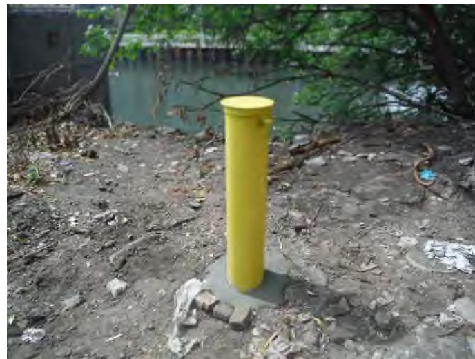
Photograph 30: View of a paired monitoring well with a stick-up protective cover.. Date: September 13, 2017.
