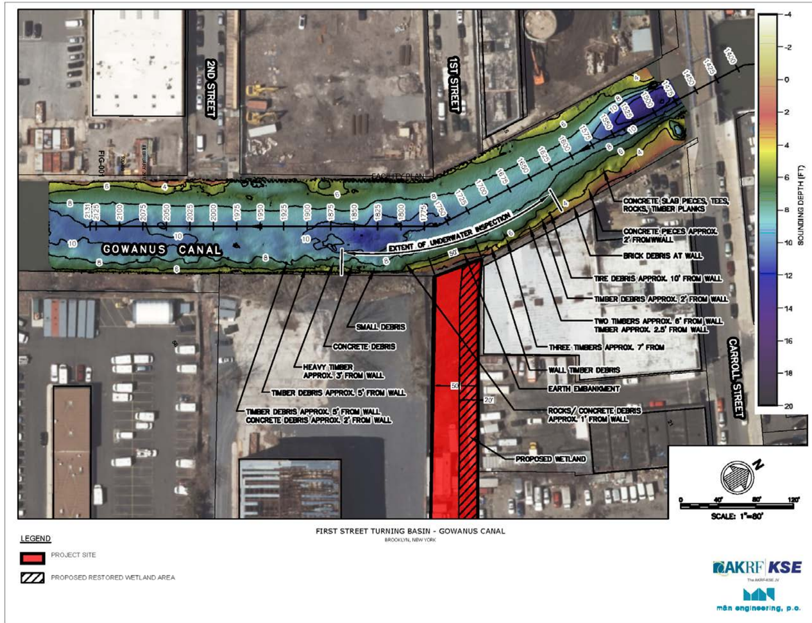
FIGURE 2 - HYDROGRAPHIC SURVEY WITH ANOMALIES IDENTIFIED
