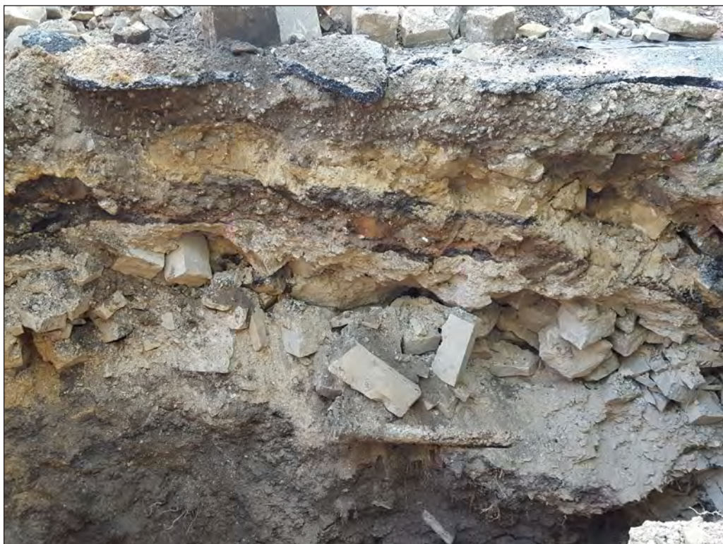
Facing west showing upper portion of western wall of TP6. Note multiple layers of loose fill and demolition debris. A 2-inch diameter pipe is located at the bottom of the photo. 23
