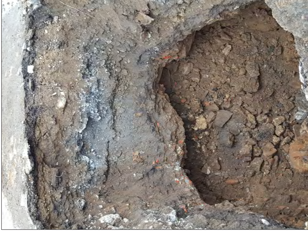
16 Facing south into TP3. Note multiple layers of fill and loose sandy fill at bottom.
