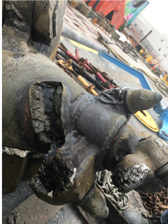
Figure 4. Photo of a Damaged Auger Head
