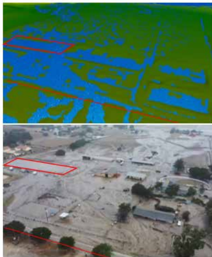
Figure 1 Top: HEC RAS model results Bottom: Drone footage
